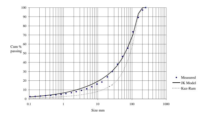
Figure 8. Predicted and measured crusher product (or SAG feed) distribution
