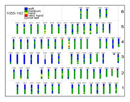
Figure 1. Blasthole geology reported by the drill monitors
