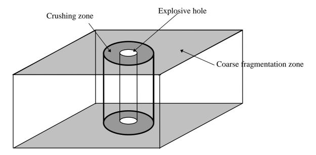
Figure 4. Schematic of the Crushed Zone Approach
